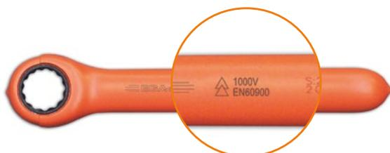
Insulated tools can be identified thanks to the marking on the insulating material. The sign should include a double triangle followed by a 1000V sign and a reference to the standard. In addition, EGA Master tools always include the product reference code and the year of manufacture for a better traceability.
